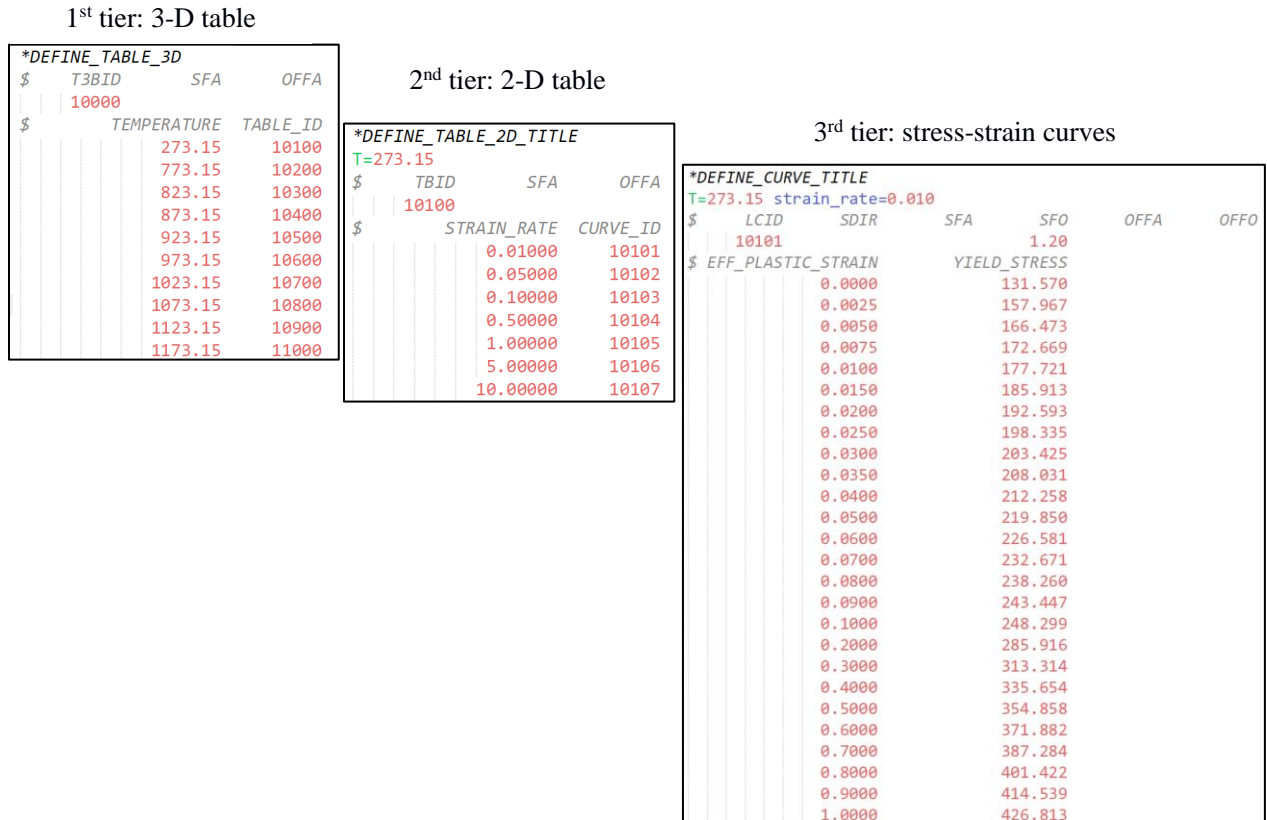
Figure 2 Example of 3-D Table characterizing rate-and-temperature-dependent hardening
