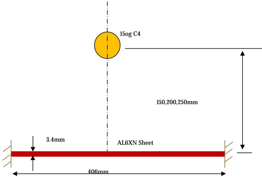
Figure 1 Sketch of the experimental set-up
