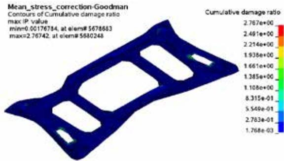
Figure 9. Cumulative damage ratio for z-acceleration PSD (using Goodman's equation for mean stress correction)
