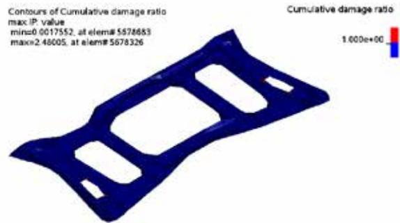
Figure 5. Safe / Failed zone for the case of z-acceleration
