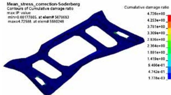
Figure 10. Cumulative damage ratio for z-acceleration PSD (using Soderberg's equation for mean stress correction)
