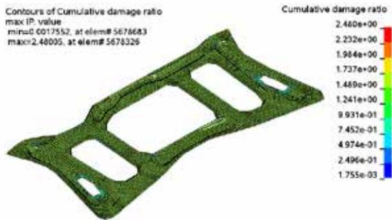
Figure 4. Cumulative damage ratio for the case of z-acceleration
