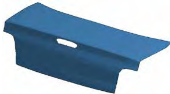
Figure 11. A trunk lid BEM model
