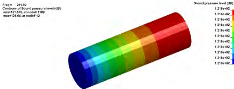
Figure 2. Sound pressure Level (dB) at frequency 211.92 Hz
