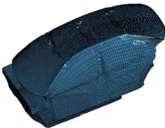
Figure 16. An auto compartment FEM model
