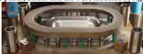
Fig. 7. Experimental setup for the double dome test.
