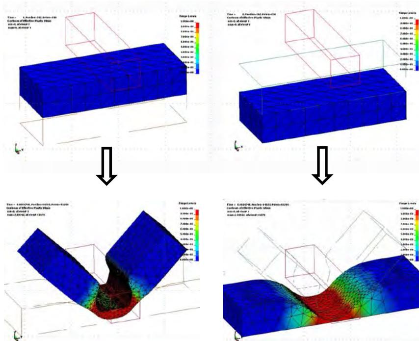
In the example shown above, there are adaptive parts: the top one contacts with a very sharp tool so that a smaller mesh size is needed to well represent the contact surface and better simulate the local large deformation; the bottom part has much smoother profile of
