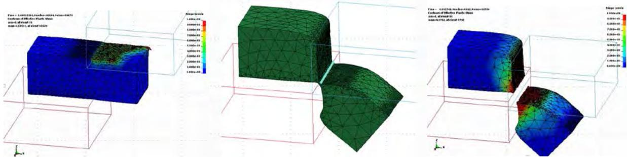
In the metal cutting simulation shown above, it can be estimated when the tool front meets the bottom die so that the additional adaptive step can be triggered for users to trim the mesh using CAD software and then continue the analysis in LS-DYNA.
